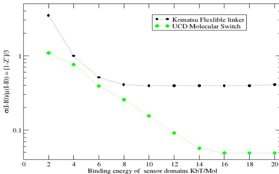
*The innovative UCD hinged peptide molecular switch has a superior signal-to-noise ratio at higher binding energies than the earlier Komatsu Flexible Linker (developed in 2011).*
